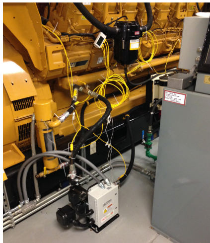
Figure 4. The test engine's right side with installed CSM and thermosiphon heater. Both heaters share a single return port using a Y-fitting.
