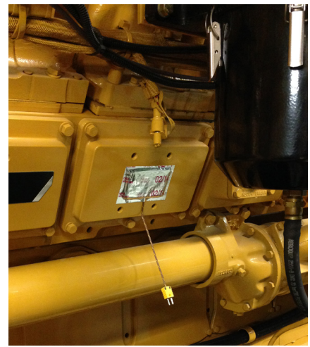
Fig 7. Thermocouple shown attached to the test engine block (above). Temperatures from all points were captured using a temperature data logger (below).
