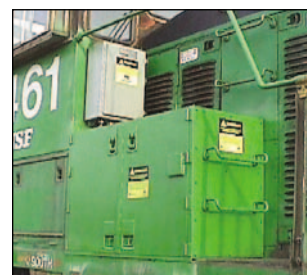
BNSF GP38 switcher 2133 (top) as equipped at Corwith Yard with an inside-mount Kim Hotstart DDHS. The unit is located at the carbody's rear (bottom left). On SW-type switchers, limited carbody space mandates that the DDHS be mounted on the walkway (bottom right).
