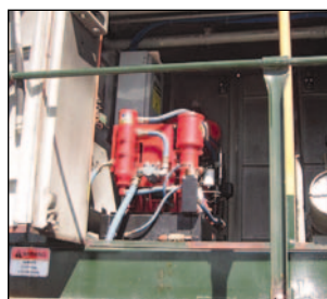
BNSF GP38 switcher 2133 (top) as equipped at Corwith Yard with an inside-mount Kim Hotstart DDHS. The unit is located at the carbody's rear (bottom left). On SW-type switchers, limited carbody space mandates that the DDHS be mounted on the walkway (bottom right).
