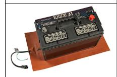
Keeping your battery heated helps to retain cranking power during cold weather. Hotstart Battery Heating Pads are placed under batteries and radiate heat within the battery box. When using Hotstart Battery Heating Pads in an insulated battery box, a thermostat is recommended to monitor temperatures to prevent overheating the battery. Battery heater pads are not recommended for nickel cadmium batteries.
