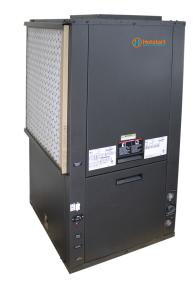
The HE Engine Heater is an energy efficient solution for maintaining optimal coolant temperature of emergency gensets. The heater utilizes heat-pump technology, sourcing heat from the ambient air at a lower energy draw than a resistive element heater.
