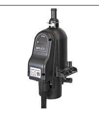
The EVRHEAT Series 20 engine heater features integrated controls and sensors to monitor the status of the heater and coolant; if an air pocket or other fault is detected, the heater deactivates power allowing for users to safely resolve the fault and reset the heater. The user screen shows at-a-glance heater operation allowing technicians to know current status. The EVR20 is the most energy efficient heater for engines up to 20 L displacement or up to 500 kW.
